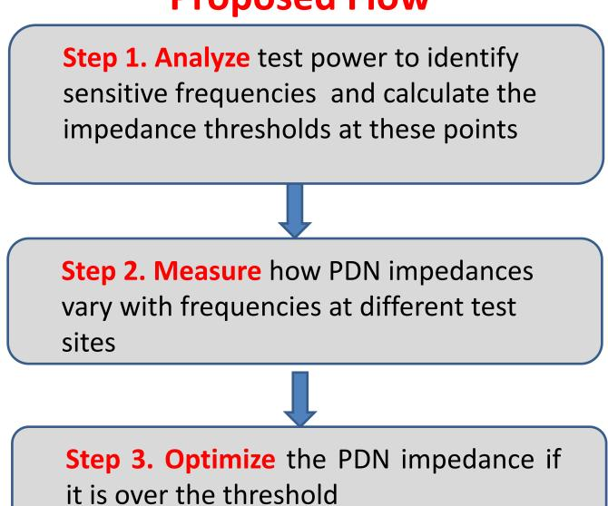
Identify the sensitive frequency points, at which the worst IR drops may happen. The following is an example of peak power analysis results based on simulation.
