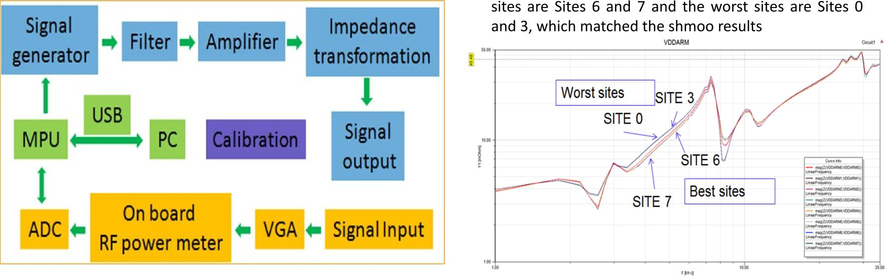
With the designed circuitry, we measure the impedance vs. the frequency. In this example, the best sites are Sites 6 and 7 and the worst sites are Sites 0
